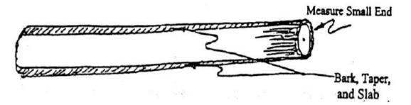
→ The diameter of a log is always measured inside the bark. This measurement is called "*diameter inside of bark*" or *d.i.b*. Use a log scale stick to measure the d.i.b. at the small end of the log.
