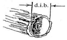
**NOTE**: The ends of logs are not always circular, so the diameter is determined by averaging the short measurement and long measurement, taken at 90 degrees from each other. Both measurements are taken through the true (geometric) center of the log, not the "center" of the log as shown by growth rings or pith.
