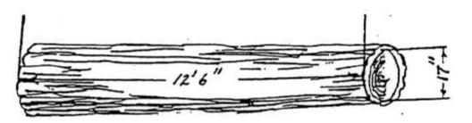
Remember, although the measured length is 12 feet plus the full trim allowance of 6 inches, the log is 12 feet in scaling length. The correct answer from the table is 17 d.i.b. x 12 ft.  $\rightarrow$  14 Decimal C volume, so it must be multiplied by 10 to give the gross board foot volume. Therefore, the correct log volume is **140** board feet.
