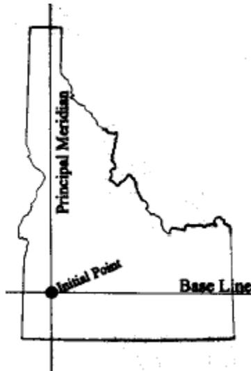
The state is subdivided by lines running at six-mile intervals, both parallel to the Base Line and to the Principal Meridian. The lines running east-west are called **Township (T)** lines and are numbered consecutively **North (N)** and **South (S)** of the Base Line. The first line north of the Base Line is *Township 1 North (T. 1 N.)* and the first line south of the Base Line is *Township 1 South (T. 1 S.)*, as illustrated below:
