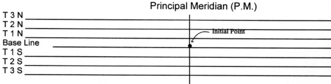
The lines running north-south at six-mile intervals are called **Range (R)** lines and are numbered consecutively **East (E)** and **West (W)** of the Principal Meridian (PM). *Range 1 East* is the first column to the right (east) of the PM. *Range 1 West* is the first column to the left of the PM, as illustrated below:
