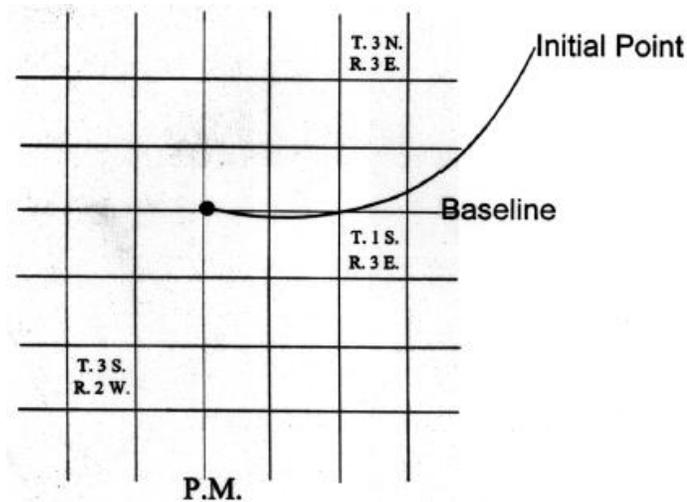
Townships (which have 6 miles per side) are further subdivided into 36 square miles called **sections**. Each section is one square mile and contains 640 acres. The following system is used to number the individual sections in a township:
